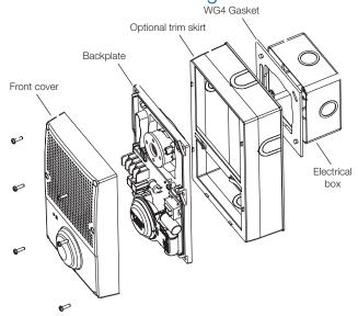
WG4 notification appliances are rated for outdoor use and are suitable for indoor or outdoor applications on walls or ceilings. For surface-mounting in outdoor or wet applications, appliances must be mounted to a 449 electrical box. In dry conditions, they are compatible with standard 4-inch square by 1½-inch deep electrical boxes. When using the optional WG4WTS or WG4RTS trim skirt, a 449 or 4-inch square by 2-1/8" deep box must be used.
