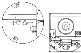
Test points indicated above are used to validate the Notification Appliance Circuit and verify device function.
