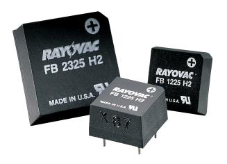
Rayovac FB batteries consist of two Lithium Carbon-monofluoride coin cells encapsulated within a glass filled polyester molded housing. The FB series of batteries are configured to allow for series or parallel interconnection between the cells.
