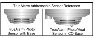
**Programmable sensitivity** of each sensor can be selected at the control panel for different levels of smoke obscuration (shown directly in percent) or for specific heat detection levels. To evaluate whether the sensitivity should be revised, the peak value is stored in memory and can be easily read (or downloaded as a report) and compared to the alarm threshold directly in percent.
