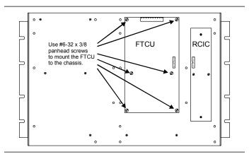
3. Secure the ASU board to the designated stand-offs in the figure below with the  $6-32 \times 3/8$  panhead screws provided.
